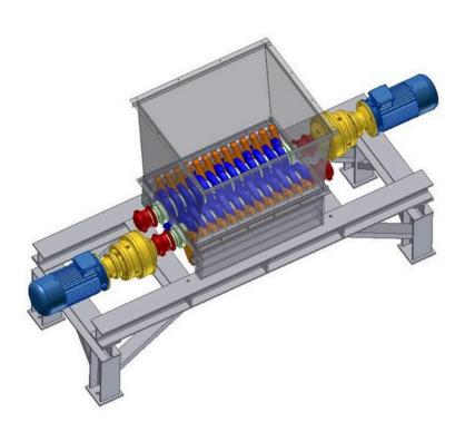
Promeco Rotor Shears Shredder has been engineered for a sharp cut for every material. Cutting discs are designed according to the material to be shred. The PRS is equipped with rotor cleaning system. The PRS is designed to shred C&I waste. The machine is equipped with two rotors with independent motors. The rotors are made of a series of hook discs that allow grasping and cutting of the material.
