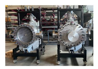
The continuous melt-filtration system PF makes possible uninterrupted extrusion, even when processing highly contaminated materials. Unlike conventional screen changers, which require extensive and constant operator attention, the PF can operate automatically.
