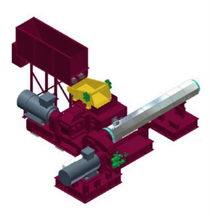
The densification & pelletizing line is made of the combination of the Promeco Extruder System PES600 + the Pellettizer Promeco PE300. The COMBO PES+PE allows the complete removal of moisture from the plastics degassing the material.
