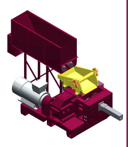
The Promeco Extruder System® (PES) produces briquettes with diameter from 60 to 100 mm.
